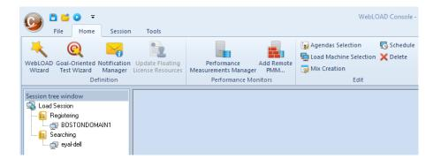
Below the load session you first add the agendas to run in the test, and for each agenda you define the Load Generator that will run it. In the example above, there are two agendas defined - Registering and Searching. Two different load generators machines will execute each agenda.
